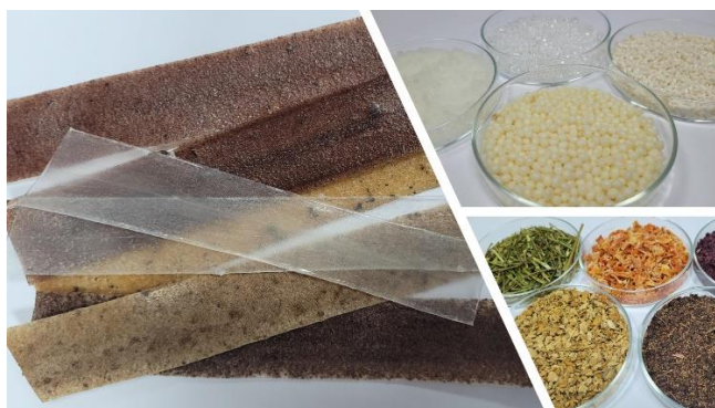
Figure 1. Biocomposite and raw materials used for their preparation (polymer granules and plant additives)
